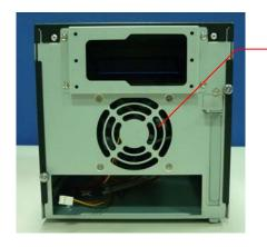
5.2 The 8cm fan at rear directly get power supply from the PSU on top, to simplify the arrangement of different cables.
