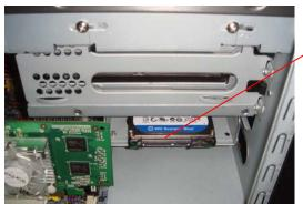
4.3 The picture shows when 2.5"HDD is installed.
