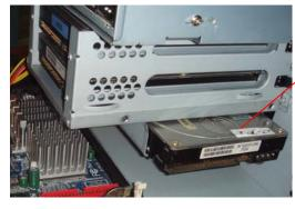
4.2 The picture shows when 3.5"HDD is installed.
