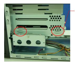
6.1 Use the cable tie that is in the accessory screw bag, arrange the cables to tie along with the chassis, to make sure air ventilation is not affected.
