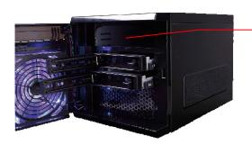
2.1 Open Front Panel; Slide in ODD, then screw the ODD into position.
