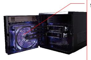
5.1, The front 12cm fan will automatically inhale cool air into the system drives when the power is on, and the heat will exit from the side panel or sucked out by the 8cm fan at rear.
