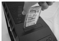
3. Pre-installed backplane is ready to use for hot plug purpose.
