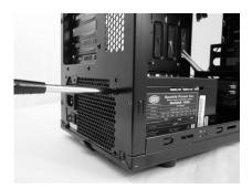
2. Simply route the cables behind the motherboard tray and part power cables with the provided cable tie.
