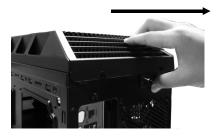
2.Install the fan with the provided screws.
