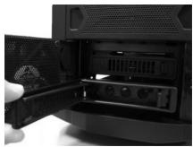
2. Attach the 3.5" drive to the tray and secure with the provided screws.
