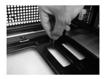
3. Align the holes of motherboard and motherboard tray, and secure the motherboard with the provided screws.
