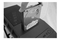
2. The docking is designed at its right size of 3.5" or 2.5".
